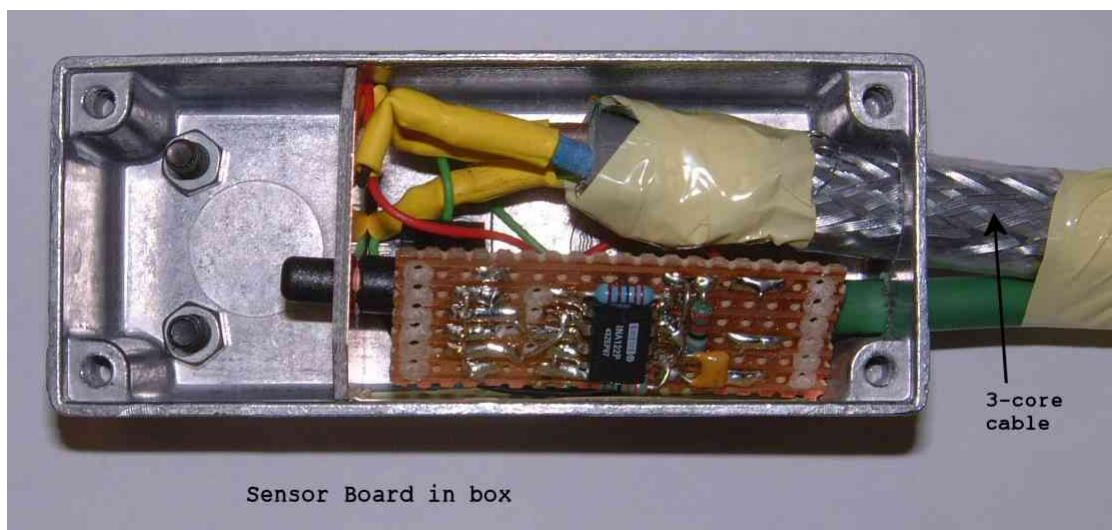
The top end of the cable connects to the 3-pin connector marked (6) in the picture of the control board. The resolution of the sensor should be approximately 1V per metre of water. This can be fine tuned later as a software variable. A dummy connector with a simple potential divider can be connected to provide a constant 1V signal when testing the controller board in the absence of a sensor module.
